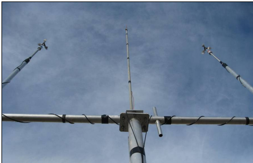
Figure B-4. Met Tower Hub Height Anemometers
