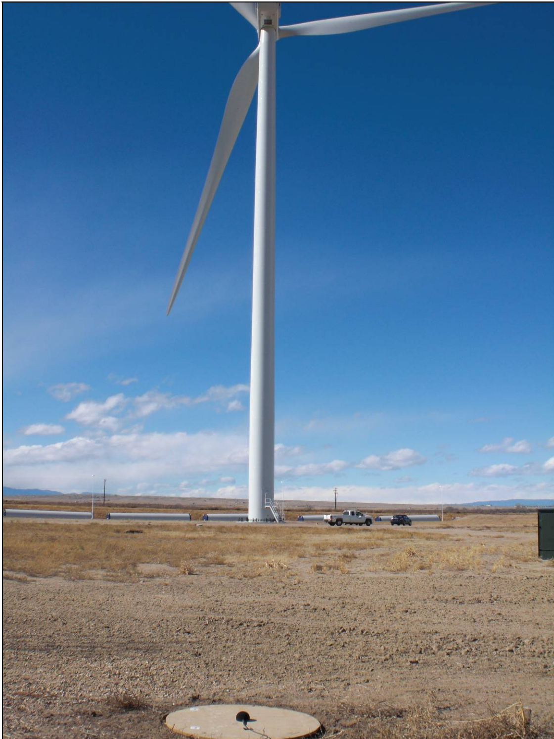
Figure B-2. Wind Turbine Under Measurement and Microphone
