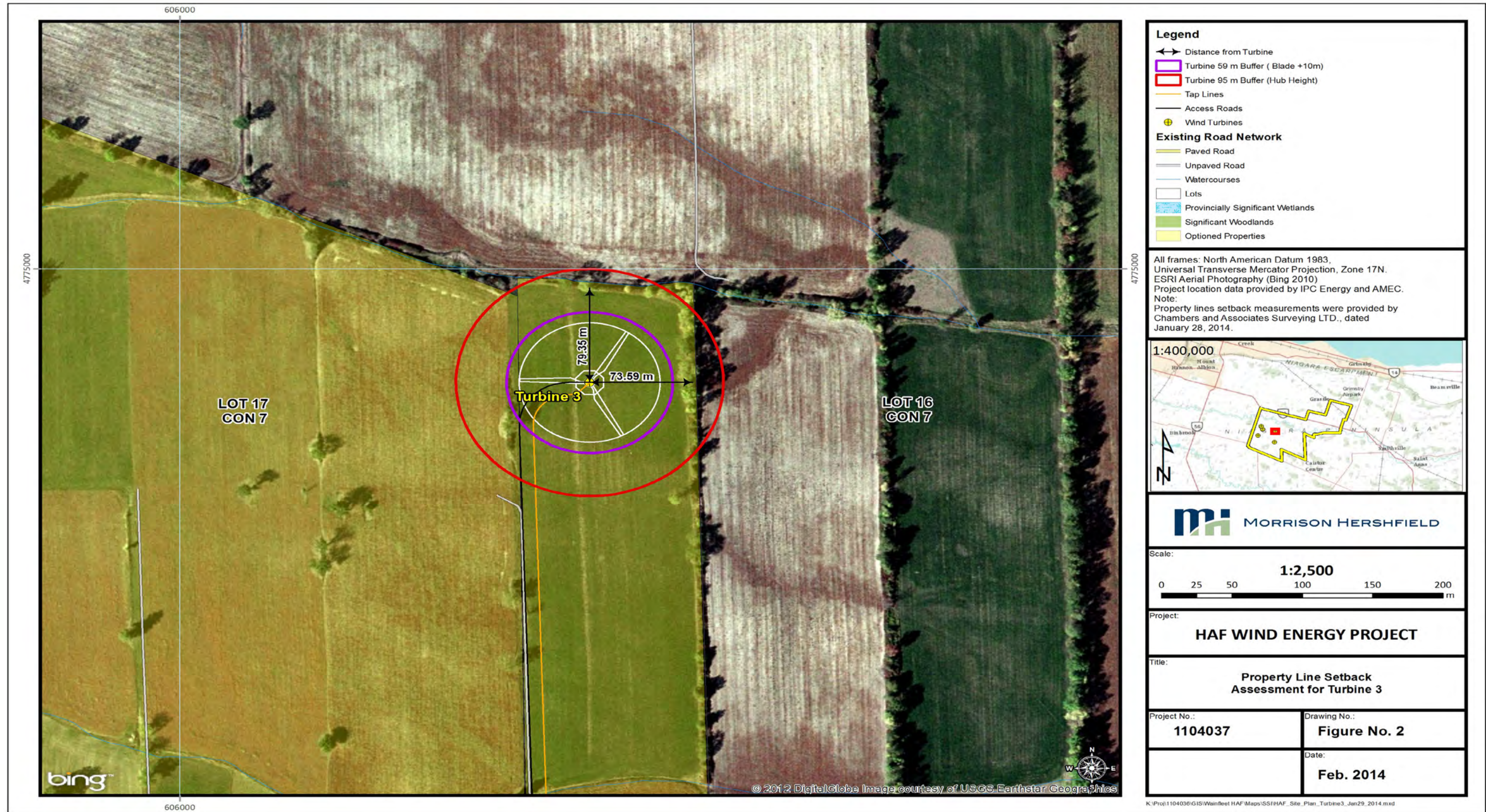
Figure 2: Property Line Setback for Turbine 3
