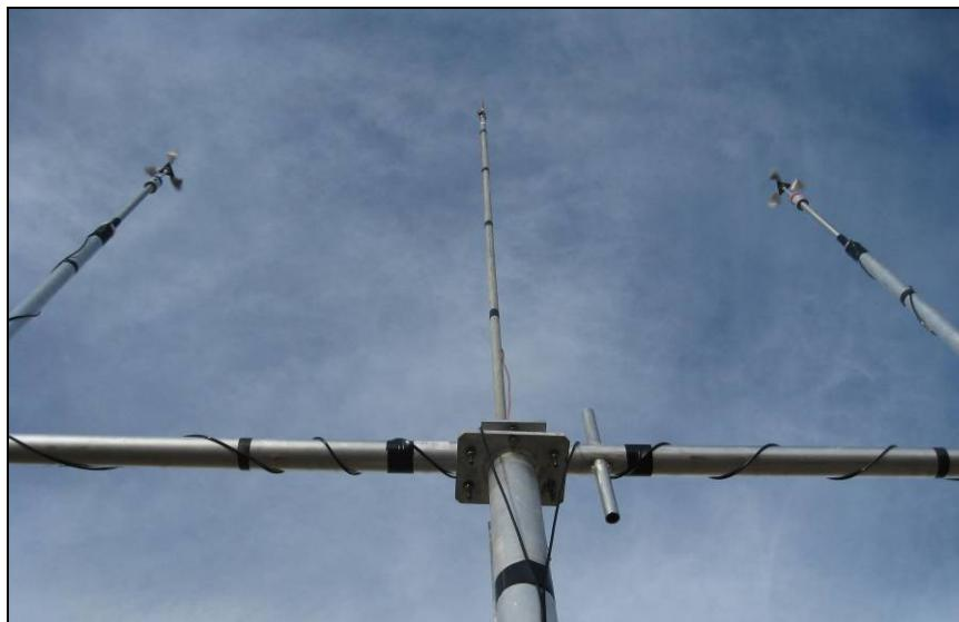
**Figure B-4. Met Tower Hub Height Anemometers**
